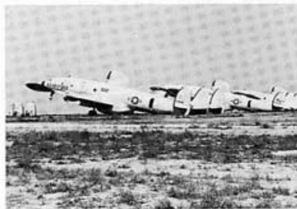
C-121 Constellations dip on their tails when the engines are removed. These aircraft were once based at Keflavik, Iceland as airborne early warning aircraft until the AWACS took over their jobs.
