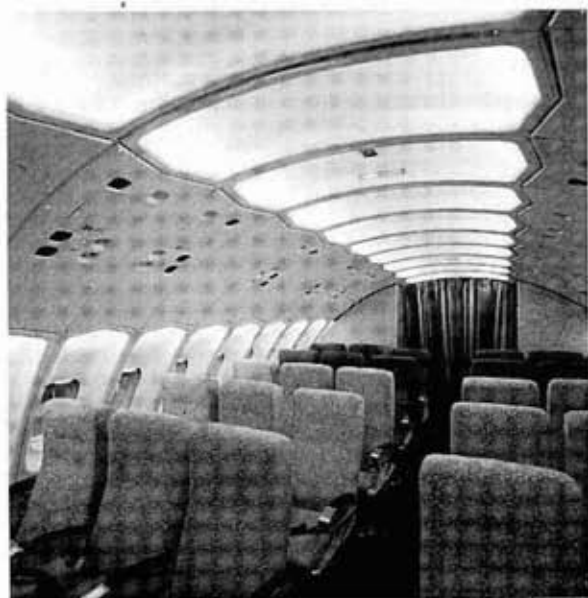
Ceiling, wall-panels, chair cover and floor-covering of synthetic material (Photo: DSM).
