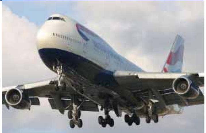
Because a single-deck wide-body fuselage was foreseen for that, to accommodate two rows of 8 ft wide standard cargo containers side-by-side, the solution for the upload was through an upward-hinging nose door. Therefore, the cockpit had to be raised and a second deck was added in the front of the aircraft and that's how the most famous feature of the 747, its hump, appeared.
